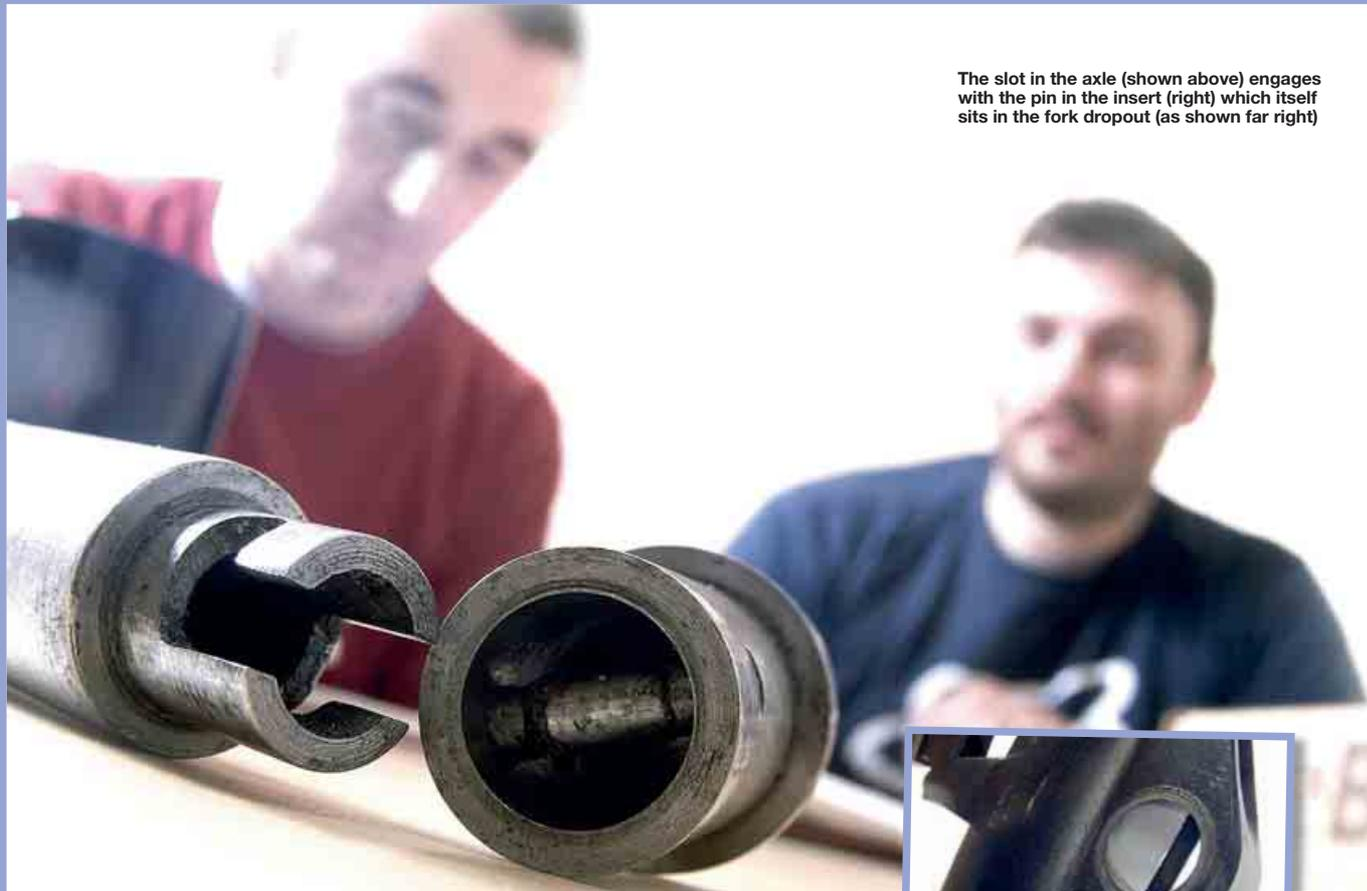
The slot in the axle (shown above) engages with the pin in the insert (right) which itself sits in the fork dropout (as shown far right)
